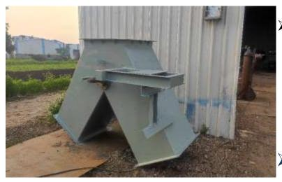
Manufactured and Supplied Motorized Diverter Gates For, Steel Industry, Power Sector & Mining.
